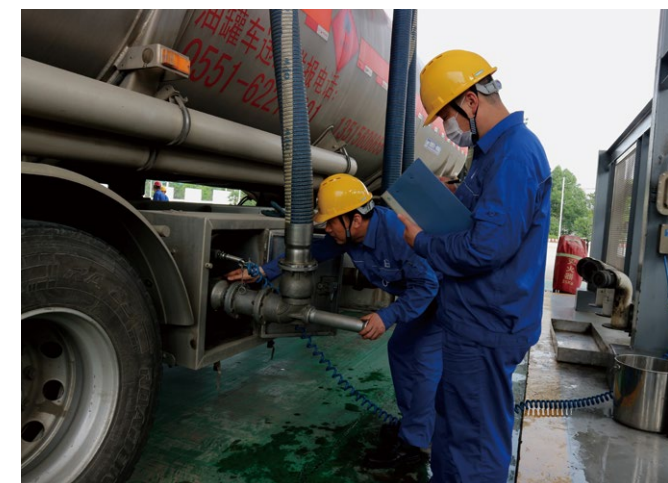
Ⓐ Safety personnel inspecting a tanker vehicle to for leakage hazards of at Feixi Oil Depot
